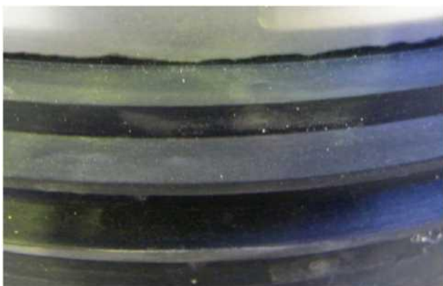
Figure 5: Sealing lips of collar H2077-1, test distance 1
