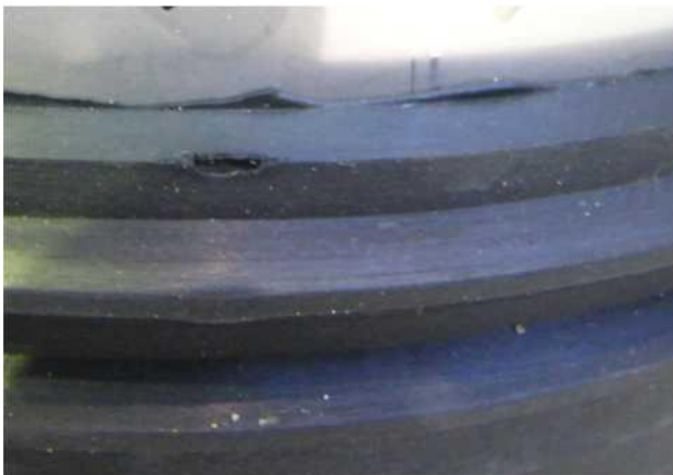
Figure 7: Alterations to the elastomer side of the collar H2077-1, test distance 2
