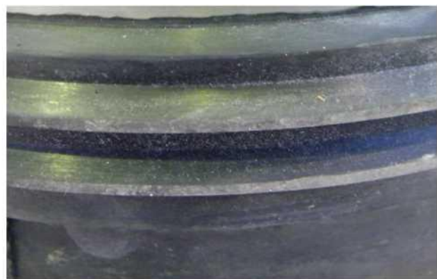
Figure 6: Sealing lips of collar H2077-2, test distance 1
