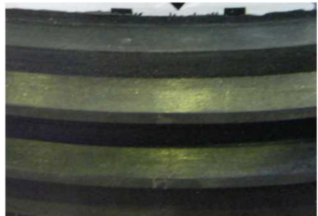
Figure 8: Sealing lips of the collar H2077-2, test distance 2
